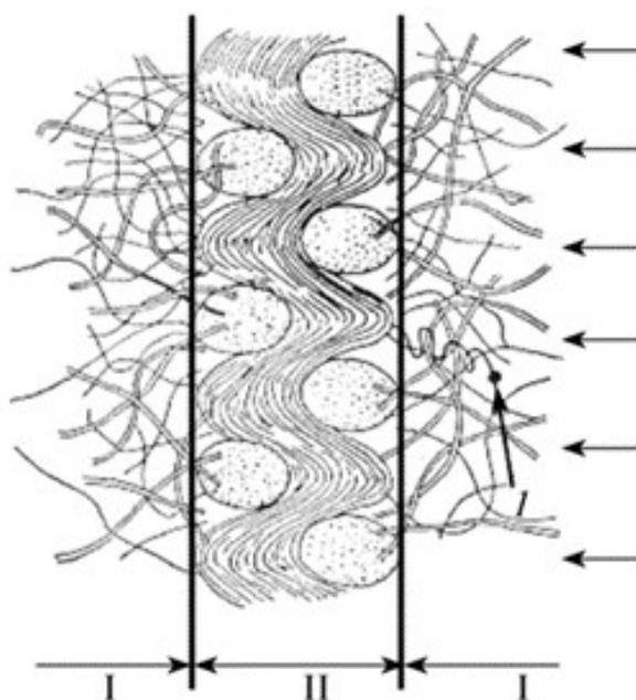
Fig.1. Cross section of the filter cloth:
