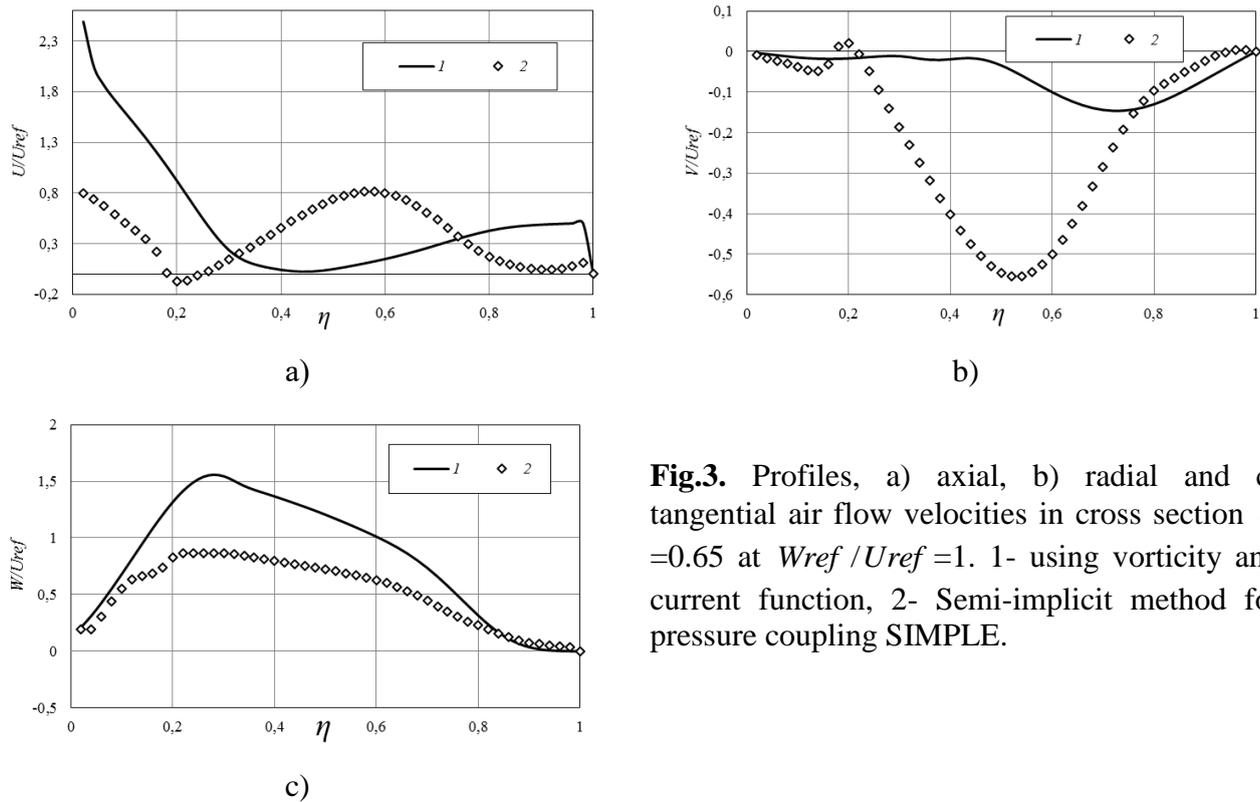
**Fig.3.** Profiles, a) axial, b) radial and c) tangential air flow velocities in cross section  $\xi = 0.65$  at  $W_{ref}/U_{ref} = 1$ . 1- using vorticity and current function, 2- Semi-implicit method for pressure coupling SIMPLE.
