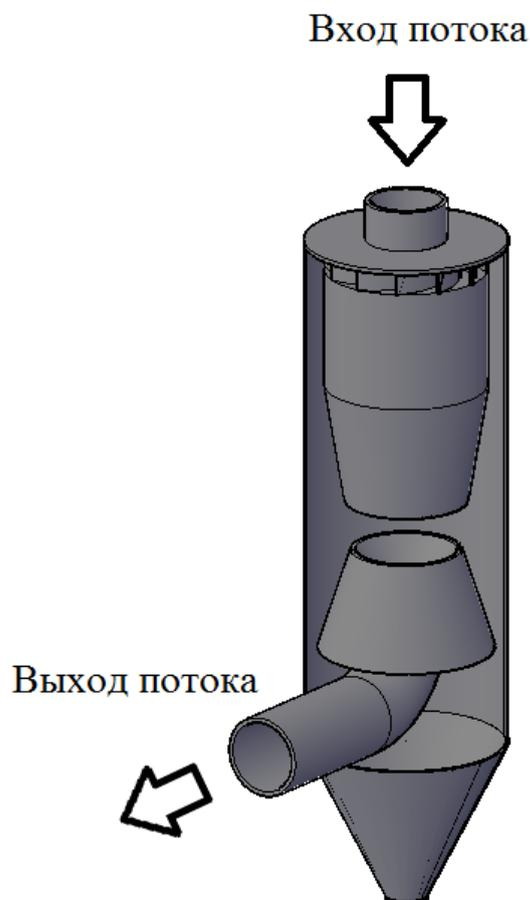
Fig. 1 Diagram of the calculated air-centrifugal separator.
