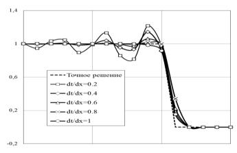
Fig. 4. The solution of the Burgers equation obtained by the Mac-Cormack scheme.
