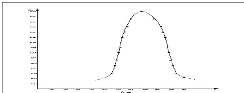
Dependence of the optical density of the complex of cobalt Yun 4- sulfo- $\beta$ -nitroso- $\alpha$ -naphthol on the tyolkin length
