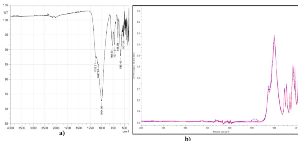
4- Image. a) Langar leucocratic granite and b) Pitov pegmatite samples sintered at 900, 1100, and 1200 °C and their IR spectra
