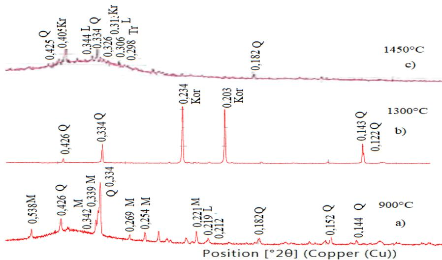
**6-Image. X-rayograms of Pitov granite samples fired at high temperatures**
