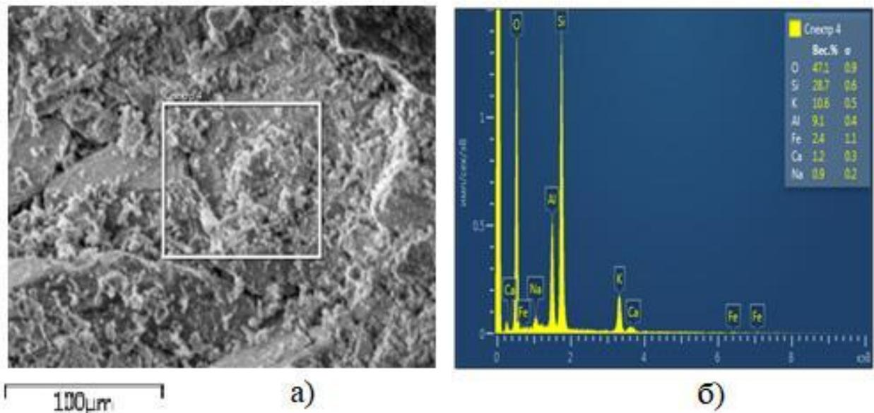
5- Image. Pitov pegmatite appearance under a scanning electron microscope
