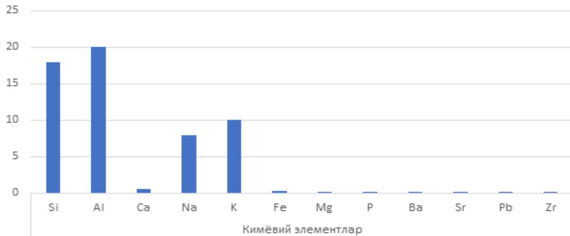
**1-Image. Diagram of the half-quantitative elemental spectral analysis of the Pitov pegmatite feldspar sample**
