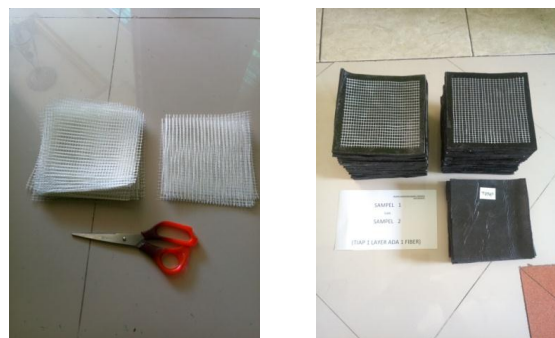
Figure 4. (a) Fiberglass cutting (b) Fiberglass layer on rubber compound layer
