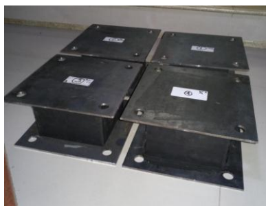
Figure 10. LCRBI-S with fiberglass and Chemlock reinforcement
