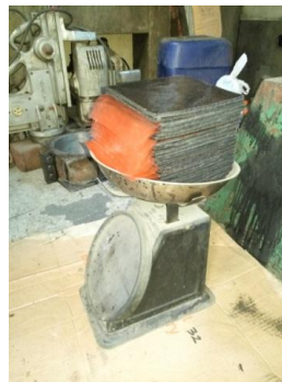
Figure 6. Weighing of rubber layers and fiberglass composites
