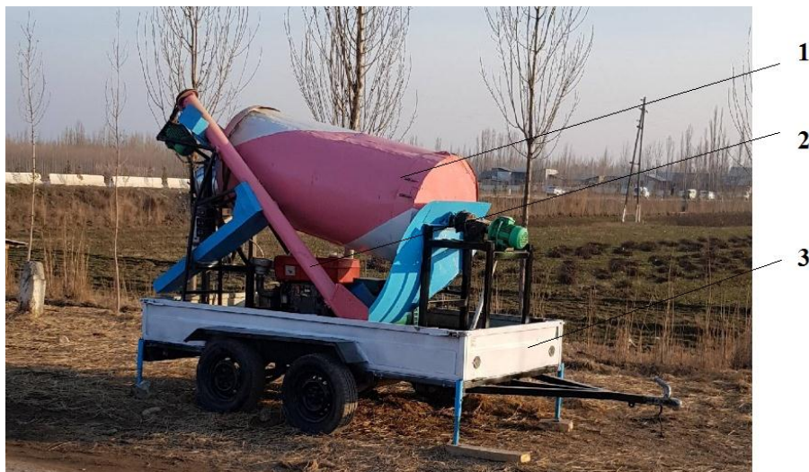
1- dryer drum; 2 screw conveyor; 3-trailer. Figure 1. Mobile paddy dryer.
