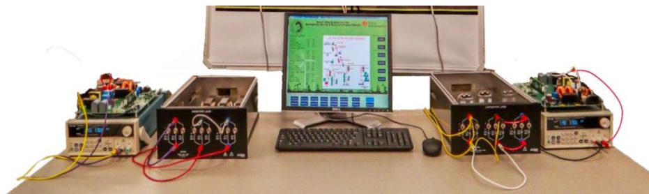
Figure-11. Microgrid Test-Layout
