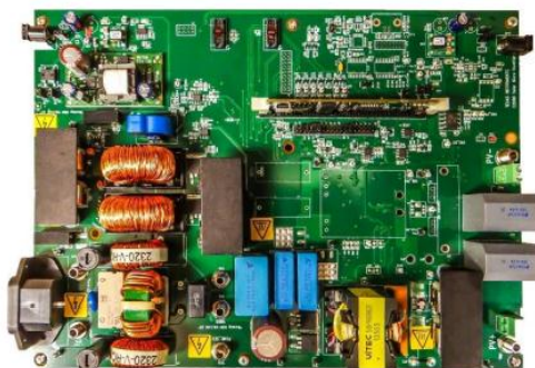
Figure-6. Grid Tie Inverter Computer Controllable Loads
