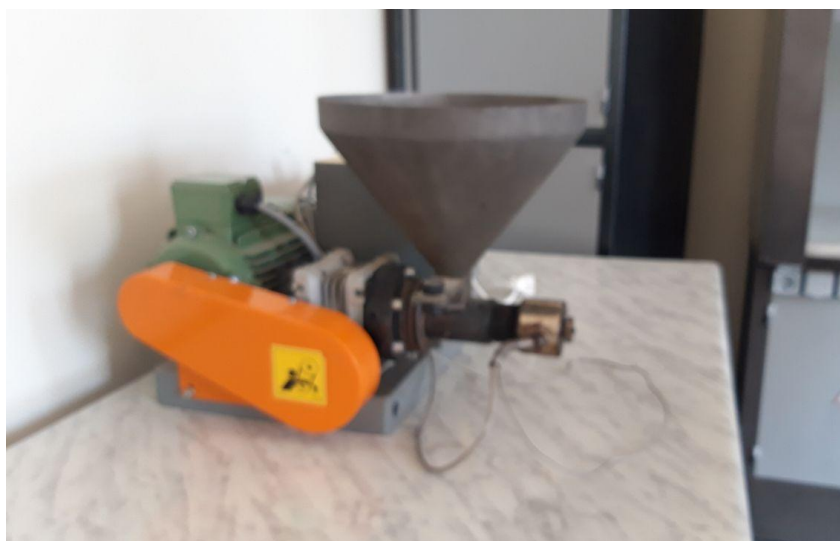
Figure 3. Laboratory device for extracting oil from grape seed by pressing method
