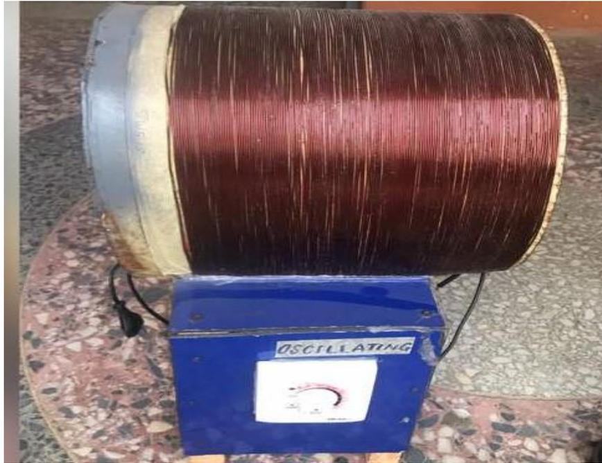
Figure 1: Solenoid for generating an oscillating magnetic field (OSMF)
