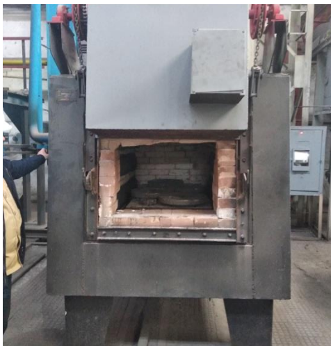
Figure 2. SNOL – 7.2/1100 muffle furnace
