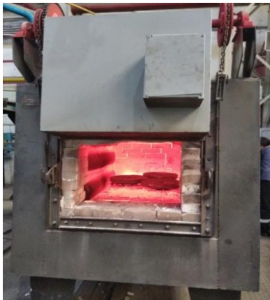
4 – picture. The process of loading the supply disc part into the furnace
