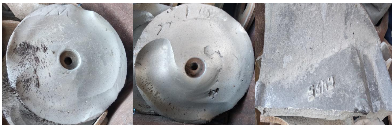
1 – picture. View of a failed provisioning disc dump
