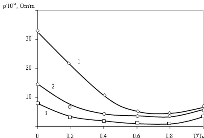
Fig. 1. Influence of the baking temperature of the carbide powder on the electrical resistivity: 1 – TN20; 2 – T14K8; 3 – VK8
