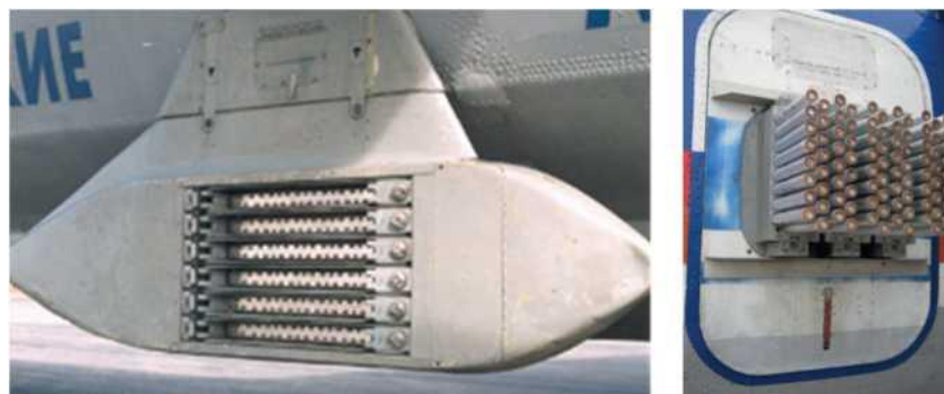
ASO-2I system with PV-26-01 squibs on An-26 (An-30) aircraft (a) and UV-26 system with SAG-26 generators on An-28 aircraft (b)
