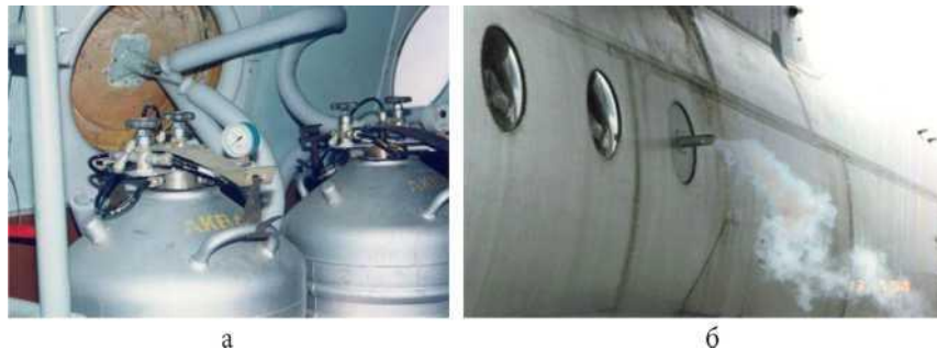
Aircraft generator of fine ice particles GMCHL-A (a), ground check GMCHL-A on AN-12 aircraft (b)
